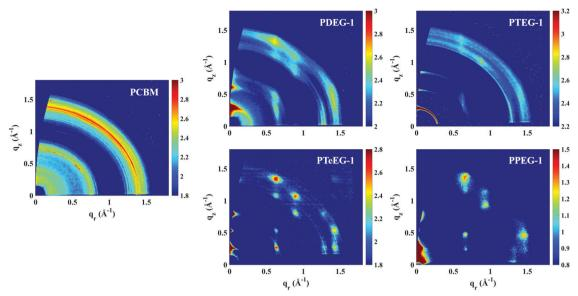
Fig. 2 GIWAXS patterns for the  $C_{60}$ -EG derivatives spin coated from chloroform solutions. The GIWAXS for a PCBM thin film is also reported for comparison. Note that the PPEG-1 sample was measured using the lab X-ray instrument, while all the others were measured at the synchrotron.
