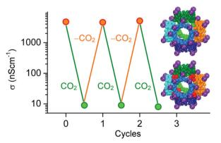
Fig. 7 Graph of the average conductivity values of CDMOF-2 as a function of the CO<sub>2</sub> concentration in N<sub>2</sub> atmosphere. The structural change of the MOF's  $\gamma$ -cyclodextrin ( $\gamma$ -CD) linker upon reaction with CO<sub>2</sub> is also shown.62
