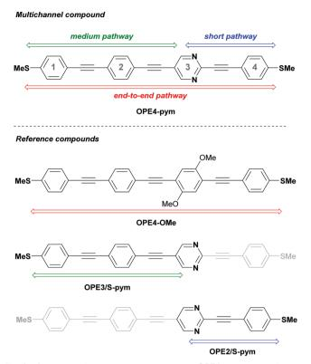
Fig. 2 Structure of multichannel compound OPE4-pym and reference compounds for each possible conduction pathway.
