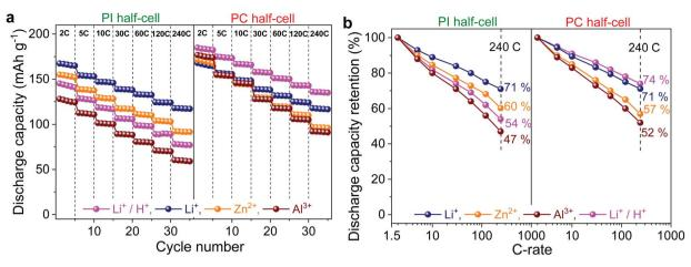
Fig. 3 (a) Discharge capacity vs. cycle number at increasing C-rates. (b) Discharge capacity retention at different C-rates. The discharge capacities at higher C-rates are normalized with respect to the discharge capacity at 2C (1C = 166 and 180 mA  $g^{-1}$  for PI and PC, respectively).
