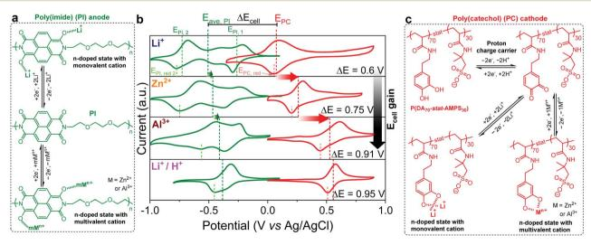
Fig. 1 (a and c) Schematic representation of the n-type redox behavior of PI (a) and PC (c) with both mono- and multivalent cations. (b) Cyclic voltammograms of PI (profiles in green) and PC (profiles in red) half-cells in unbuffered aqueous electrolytes containing different charge carriers, i.e., Li<sup>+</sup>,  $Zn^{2+}$ ,  $Al^{3+}$ , and Li<sup>+</sup>/H<sup>+</sup> (top to bottom). The CVs were recorded at 10 mV s<sup>-1</sup> in a standard three-electrode configuration.
