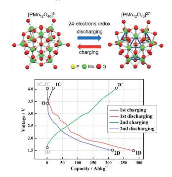
Fig. 5 Structures of POMs  $[PMo_{12}O_{40}]^{3-}$  and  $[PMo_{12}O_{40}]^{27-}$ . Charging and discharging curves of a POM/Li battery. Extracted from ref. 127.
