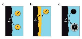
Fig. 3 Schematic representation of the electron transfer phenomena for the different types of RFB: all liquid (a), metal hybrid battery (b) and semi-solid (c).
