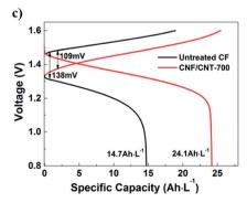
Fig. 11 SEM image of (a) untreated CF, (b) CNF/CNT grown CF surface. (c) Charge-discharge voltage profiles of VRFB employing untreated and CNF/CNT-T electrodes at 40 mA cm<sup>-2</sup>. Extracted from ref. 355.
