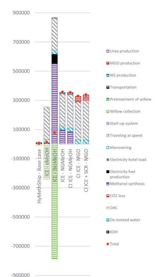
Fig. 5 Process contribution to climate change (GWP100) for all cases. Unit kg CO<sub>2</sub> equivalents. Presented per round trip between Gothenburg and Kiel on a RoPax vessel.
