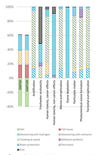
Fig. 4 The contribution to each impact category presented per process in the life cycle of the HyMethShip concept without background electricity production processes. The results are for scenario A in Fig. 2.
