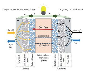
Fig. 2 Schematic representation of an alkaline anion exchange membrane fuel cell (AAEMFC) adapted from ref. 14 with permission from [Elsevier], copyright [2020].
