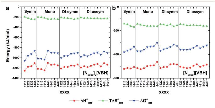
Fig. 4 DFT calculated lattice energy profiles of the  $[N_{xxxx}]_y[VBH]$  active materials in the (a) +4 (where y=2) and (b) +5 (where y=1) states. Crystals are grouped into unsubstituted (Symm), mono-substituted (Mono), symmetric disubstituted (Di-symm), and asymmetric disubstituted (Di-asymm) cations and a group is arranged by increasing cation size.
