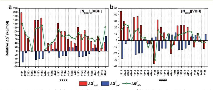
Fig. 6 Free energies of sublimation  $(\Delta G_{\text{sub}}^*)$ , solvation  $(\Delta G_{\text{sol}}^*)$  in MeCN, and dissolution  $(\Delta G_{\text{dis}}^*)$  in MeCN of the  $[N_{\text{XXXX}}]_y[\text{VBH}]$  active materials in the (a) +4 (where y=2) and (b) +5 (where y=1) states relative to the free energies of  $[N_{4444}]_2[\text{VBH}]$  and  $[N_{4444}][\text{VBH}]$ , respectively.
