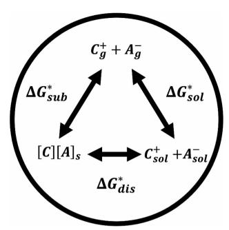
Fig. 2 Schematic representation of the thermodynamic cycle for the dissolution of [cation][VBH] complexes. The free-energy of dissolution  $(\Delta G_{\mathrm{dis}}^*)$  determines the solubility of the complex and results from the interplay between the free energy of sublimation  $(\Delta G_{\mathrm{sub}}^*)$  and that of the stabilizing solute–solvent interactions in solution  $(\Delta G_{\mathrm{sol}}^*)$ .
