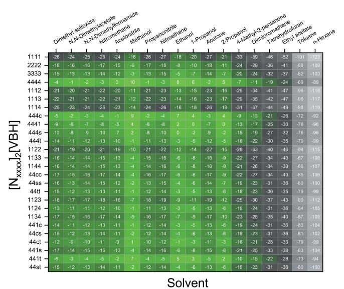
Fig. 7 Heat map of  $log(S_0)$  for  $[N_{xxxx}]_2[VBH]$  in different solvents. Solubilities were taken relative to the solubility of  $[N_{4444}]_2[VBH]$  in MeCN. Green cells indicate better or comparable solubilities with respect to  $[N_{4444}]_2[VBH]$  in MeCN.
