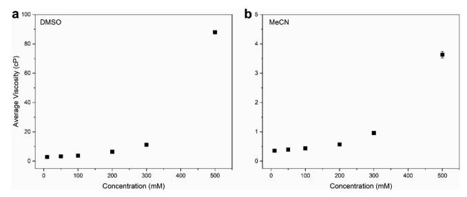
Fig. 9 Viscosity measurements of  $[N_{4444}]_2[VBH]$  in (a) DMSO and (b) MeCN at 0.01 M, 0.05 M, 0.1 M, 0.2 M, and 0.5 M concentrations. All experiments were performed using a viscometer at room temperature (25 °C).
