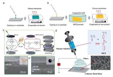
Fig. 9 Schematic illustration of membrane fabrication methods. (a) Casting method. (b) NIPS phrase separation. (c) In situ polymerization. Reproduced with permission.94 Copyright 2020, American Chemical Society. (d) Electrospinning technique. Reproduced with permission.96 Copyright 2017 Wiley
