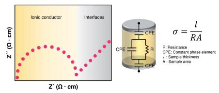
Fig. 10 Ionic conductivity characterization. Representative Nyquist plot of an ionic conductor sandwiched with blocking electrodes (left) and its equivalent circuit model for ionic conductivity measurement (right).
