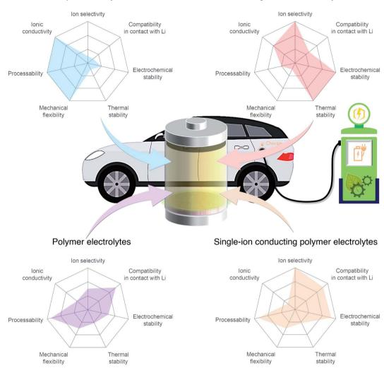
Fig. 1 Performance of different electrolyte materials. Radar plots of the properties of liquid electrolytes, inorganic solid electrolytes, polymer electrolytes, and single-ion conducting polymer electrolytes.
