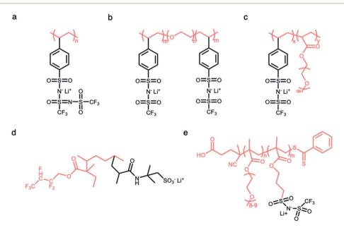
Fig. 6 Polymer matrices for constructing SIC polymers. Chemical structures of SIC polymer electrolytes with (a and b) linear polymer matrices and (c-e) branched polymer matrices. Black: anion and Li<sup>+</sup> cation; pink: polymer matrices.
