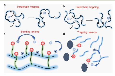
Fig. 11 Ion transport in a polymer electrolyte. (a) Intrachain hopping, (b) interchain hopping, (c) anionic site-to-site hopping, and (d) cation diffusion, while anions are trapped.
