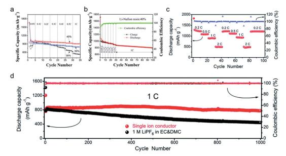
Fig. 19 Performance in Li-S batteries. The rate performance (a) and the cycling behavior (b) of the Li|PC-Li-Nafion membrane|C-S cells. (a and b) are reproduced with permission.<sup>161</sup> Copyright 2017, Elsevier. (c) Rate performance of Li|PEMA-graft-LiATFSI|S@PAN cells at various C rates and (d) cycling performances at 1C for 1000 cycles. (c and d) are reproduced with permission. 162 Copyright 2018, Royal Society of Chemistry.
