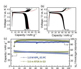
Fig. 5 Galvanostatic charge—discharge curves of KVPP electrodes in K cells filled with different electrolytes at C/20 rate in 2.0–4.5 V: (a) 1 mol dm $^{-3}$  KPF $_6$ /EC : PC (1 : 1 v/v) electrolyte and (b) 5.6 mol kg $^{-1}$  KFSA/ triglyme (G3) electrolyte. (c) Comparison of discharge capacity and coulombic efficiency of the two different electrolyte cells.
