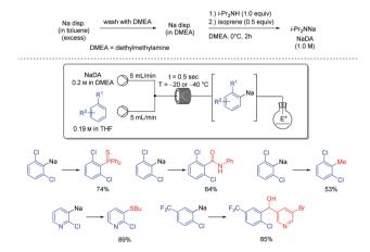
Scheme 18 Generation of aryl- and heteroaryl-sodium intermediates in continuous flow.
