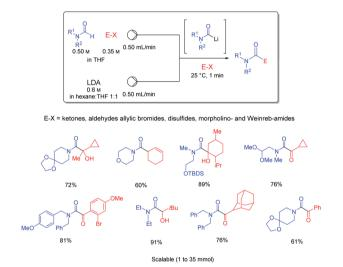
**Scheme 17** Barbier reactions in continuous flow involving an *in situ* generation of carbamoyllithium derivatives.
