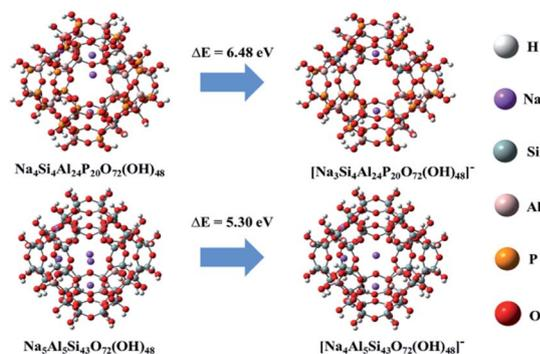
Fig. 5 Molecular structures of two neutral  $Na_5Al_5Si_{43}O_{72}(OH)_{48}$  and  $Na_4Si_4Al_2P_{20}O_{72}(OH)_{48}$  clusters and the binding energy of  $Na^+$  in the center of elliptical *s8rs* in two clusters.
