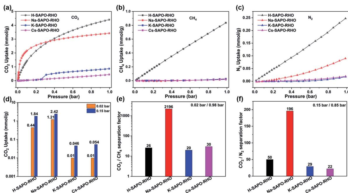
Fig. 4 Comparison of the (a) CO<sub>2</sub>, (b) CH<sub>4</sub>, and (c) N<sub>2</sub> adsorption isotherms of all SAPO-RHOs at 298 K between 0 and 1 bar; (d) comparison of the CO<sub>2</sub> uptake for all the SAPO-RHOs under 0.02 and 0.15 bar at 298 K respectively; (e) CO<sub>2</sub>/CH<sub>4</sub> separation factors at 0.02/0.98 bar and (f) CO<sub>2</sub>/N<sub>2</sub> separation factors at 0.15/0.85 bar at 298 K for all the SAPO-RHOs.
