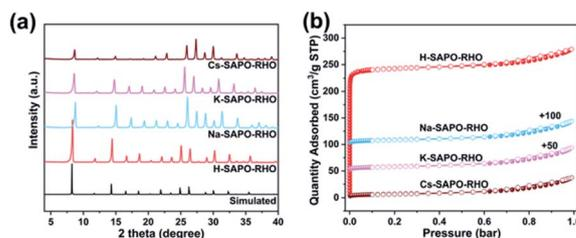
Fig. 1 (a) Simulated XRD pattern of SAPO-**RHO**s and experimental ones of the calcined M-SAPO-**RHO**s; (b) N<sub>2</sub> adsorption/desorption isotherms of the calcined SAPO-**RHO** (H-SAPO-**RHO**) and M-SAPO-**RHO**s (M = Na, K, and Cs) at 77 K.
