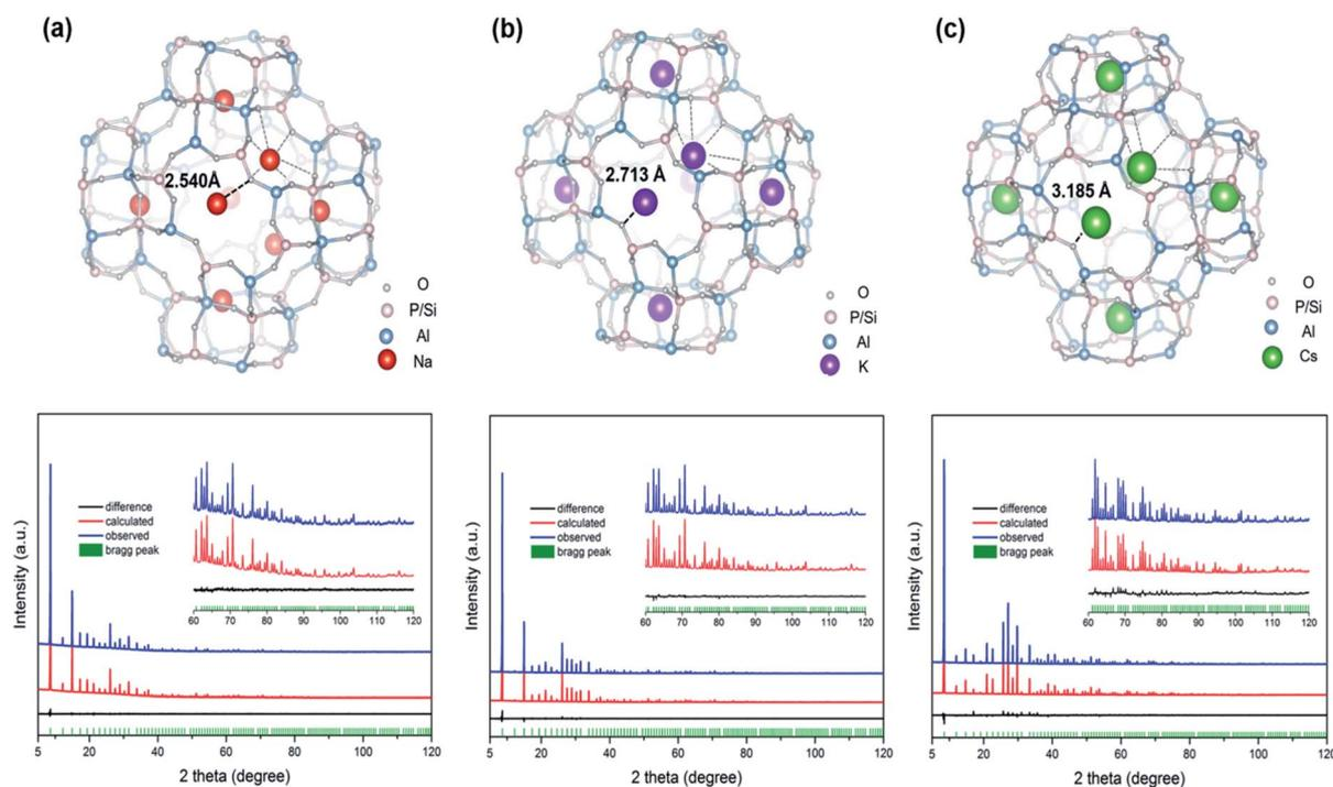
Fig. 3 Crystallographic structures of (a) de-Na-SAPO-RHO, (b) de-K-SAPO-RHO, and (c) de-Cs-SAPO-RHO and their corresponding final Rietveld refinement plots. The observed, calculated, and difference curves are in blue, red, and black, respectively. The vertical bars indicate the positions of the Bragg peaks ( $\lambda = 1.5406 \text{ \AA}$ ).
