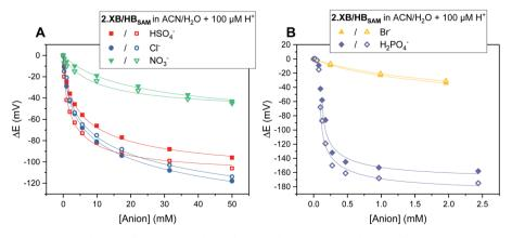
Fig. 5 Cathodic voltammetric shifts of 2.XB<sub>SAM</sub> (filled symbols) and 2.HB<sub>SAM</sub> (empty symbols) in ACN/H<sub>2</sub>O 99 :  $1 + 100 \mu$ M H<sup>+</sup> upon titration with various anions. Solid lines represent fits to a 1 : 1 host–guest Nernst model (eqn (2)). Note the different *x*- and *y*-axis scaling for both graphs.
