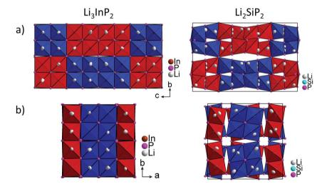
Fig. 5 Comparison of the crystal structures of Li<sub>3</sub>InP<sub>2</sub> (left) and Li<sub>2</sub>SiP<sub>2</sub> (right). (a) The unit cell in a direction. (b) The unit cell in c direction. The InP<sub>4</sub> and SiP<sub>4</sub> tetrahedra are shown in blue and red. Both structures exhibit two independent diamond-like networks of T2-supertetrahedra. The different networks are drawn in blue and red, respectively.
