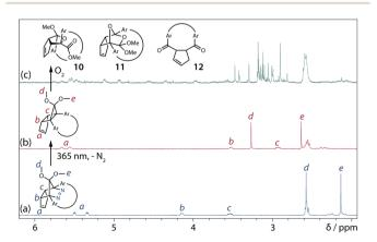
Fig. 4 In situ <sup>1</sup>H NMR (400 MHz) analysis of the photoreaction of AZ3b (4.47 mM in degassed C<sub>6</sub>D<sub>6</sub>). <sup>1</sup>H NMR spectrum of (a) AZ3b before irradiation; (b) trans-CP3b after irradiation with a 365 nm LED lamp for 90 s at 298 K under nitrogen atmosphere; and (c) trans-CP3b decomposition upon exposure to air for 3 min.
