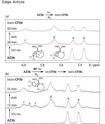
Fig. 5 In situ  $^1$ H NMR (400 MHz) analysis of the N $_2$  loss of AZ3b in degassed toluene- $d_8$  at 199 K with Nd:YAG laser irradiation ( $\lambda_{\rm emi}=355$  nm, 30 mJ). (a) Direct irradiation of AZ3b (6.49 mM); (b) Irradiation of AZ3b (0.60 mM) in the presence of benzophenone (9.32 mM).
