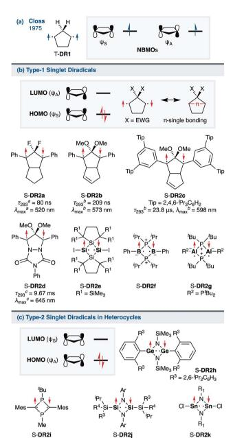
Scheme 1 (a) Pioneering work of Closs; (b) Type-1 and (c) Type-2 localised singlet diradicaloids in (hetero)cyclobutane and -pentane systems. The lifetime  $\tau_{293}$  and maximum absorption wavelength  $\lambda_{\text{max}}$  were determined in  ${}^an$ -pentane,  ${}^b$ benzene, or  ${}^c$ toluene.
