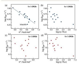
Fig. 10 Correlations between the rate constant  $\log k_{\rm CP}$  and the solvent polarity ( $\pi^*$ ) and viscosity ( $\eta$ ) for (a and b) S-DR2b and (c and d) S-DR3b.
