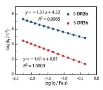
Fig. 9 Dependence of the solvent thermal fluctuation rate constant  $\log k_{\rm f}$  calculated by eqn (2) on the viscosity of GTA.  $k_{\rm Ac}$  and  $k_{\rm GTA}$  were calculated from the Eyring plot.
