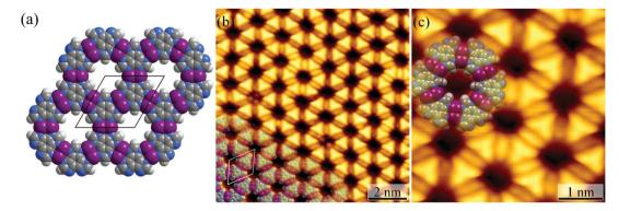
Fig. 3 (a) MM simulated structure of [Ag<sub>3</sub>btim]. (b) The large-scale (U = 1.6 V, I = 100 pA) and (c) high-resolution (U = 0.08 V, I = 1.54 nA) STM image of [Ag<sub>3</sub>(btim)] on Ag(111) surfaces. The unit cell is indicated in black/white in (a)/(b). Molecular models are superimposed on the respective image.
