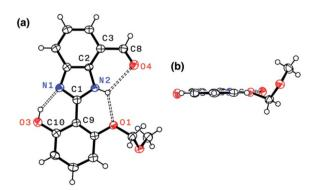
Fig. 6 X-ray structure of 4 as ORTEP diagrams with thermal ellipsoids at the 50% probability level: (a) face-on and (b) edge-on views. Selected interatomic distances (Å) of the hydrogen bonds (dashed lines):  $N1\cdots O3$ , 2.568(3);  $N2\cdots O1$ , 2.634(4);  $N2\cdots O4$ , 2.901(3).
