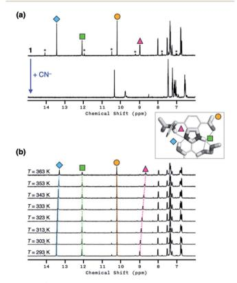
Fig. 11 (a)  $^1$ H NMR spectra of 1 (4.0 mM) prior to (top) and after (bottom) the addition of NaCN (10 equiv.) in DMSO- $d_6$  at T=298 K. Asterisks indicate the resonances of the minor tautomer which is less than 10% based on the peak integration values. (b) Variable-temperature  $^1$ H NMR spectra of 1 (4.0 mM) in DMSO- $d_6$  at T=293-363 K.
