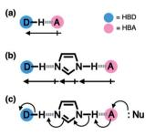
Fig. 1 Schematic representation of (a) a simple HBD–HBA pair and (b) cascade hydrogen bonding with an amphoteric proton mediator, such as imidazole, between a widely separated pair of HBD and HBA to create a larger net additive dipole to promote the addition/substitution reaction shown in (c).
