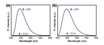
Fig. 7 Emission spectra ( $\lambda_{exc}=343$  nm) of (a) **3** (0.100 mM) prior to (black dashed lines) and after treatment with NaCN (25 equiv., blue line) or Et<sub>3</sub>N (25 equiv., gray line), and (b) **4** (0.100 mM) prior to (black dashed lines) and after treatment with NaCN (25 equiv., blue line) or Et<sub>3</sub>N (25 equiv., gray line) in DMSO at T=298 K.
