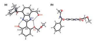
Fig. 9 X-ray structure of  $\bf 1$  as ORTEP diagrams with thermal ellipsoids at the 50% probability level: (a) face-on and (b) edge-on views. Selected interatomic distances (Å) of the hydrogen bonds (dashed lines): N1···O3, 2.5431(1); N2···O1, 2.62995(9); N2···O4, 2.9007(1).
