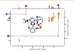
Fig. 12 Partial 2D-COSY contour plot of 1 (4.0 mM) treated with NaCN (10 equiv.) in DMSO- $d_6$  at T=298 K. The corresponding 1D NMR spectrum is shown along the ordinate. Inset: DFT (B3LYP-D3/6-31G(d,p)) energy-minimized structure of the cyanohydrin adduct of 1.
