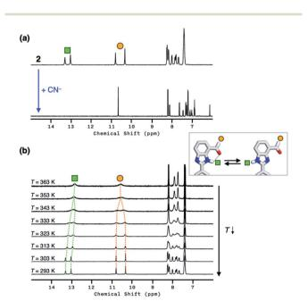
Fig. 5 (a)  $^{1}$ H NMR spectra of 2 (4.0 mM) prior to (top) and after (bottom) the addition of NaCN (10 equiv.) in DMSO- $d_6$ ; T=298 K. (b) Variable-temperature (VT)  $^{1}$ H NMR spectra of 2 (4.0 mM) in DMSO- $d_6$  measured at T=293-363 K.
