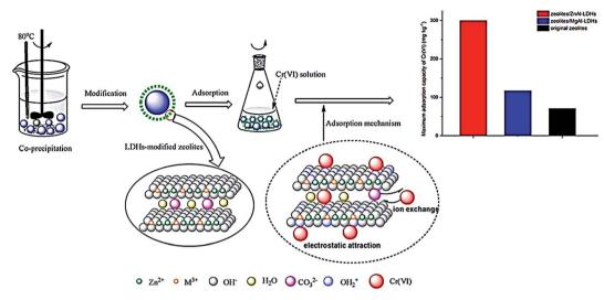
Fig. 17 Removal difference of  $Cr^{6+}$  by modified zeolites coated with MgAl and ZnAl-layered double hydroxides, adapted with permission from ref. 170, copyright, Elsevier, 2021.
