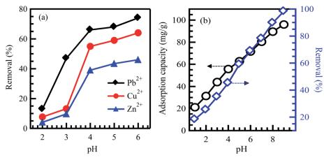
Fig. 2 Effect of initial solution pH on the adsorption of (a)  $Pb^{2+}$ ,  $Cu^{2+}$  and  $Zn^{2+}$  on modified crosslinked cellulose/sodium alginate adsorbent, reproduced with permission from ref. 40, copyright, Royal Society of Chemistry, 2018; and (b) MO dye on functionalized MWCNTs, reproduced with permission from ref. 41, copyright, Springer, 2019.
