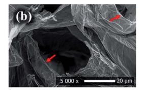
Fig. 13 SEM images (a and b) of rGO showing its unique layered structure, adapted with permission from ref. <sup>117</sup>, copyright, American Chemical Society, 2021.
