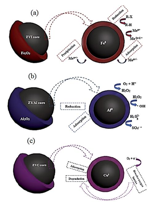
Fig. 21 Nano zero-valent iron (a) aluminum (b), and copper (c) core-shell structures with different mechanisms of contaminants removal.
