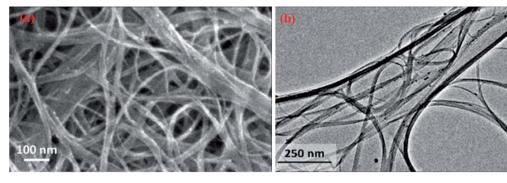
Fig. 8 SEM (a) and TEM (b) images showing the morphology of SWCNTs, adapted with permission from ref. 91, copyright, Elsevier, 2016.
