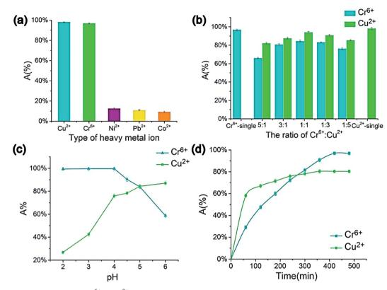
Fig. 11 Impacts of metal ions' type (a) Cr<sup>6+</sup> to Cu<sup>2+</sup> ratio, (b) pH, (c) adsorption time, and (d) on the metal ions' adsorption efficiency (composite tablet adsorbed with 10 mg L $^{-1}$  concentration under 40 °C temperature for 600 min in 4.5 pH, 5 mL of metal ion agueous solution (1 mg L $^{-1}$ ), 130 rpm), adapted with permission from ref. 104, copyright, Elsevier, 2021.
