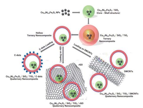
Fig. 20 Schematic presentation of the steps used to prepare CNFST composite matrix loaded with C-dots, rGO, and SWCNTs, adapted from ref. 204 with copyright permission from Elsevier, 2020.
