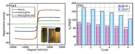
Fig. 15 (a) Magnetic properties of the prepared composite, (b) reusability of the prepared composite for the adsorption of CIP and  $Cu^{2+}$ , adapted with permission from ref. 122, copyright, Elsevier, 2021.
