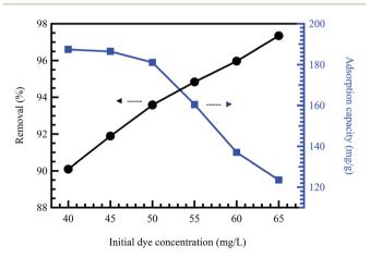
Fig. 5 Effect of initial MB concentration onto ZnCl<sub>2</sub> corn husk AC adsorbent at pH = 4, and adsorbent dose =  $0.3 \text{ g L}^{-1}$ , reproduced with permission from ref. 55, copyright, Hindawi, 2013.
