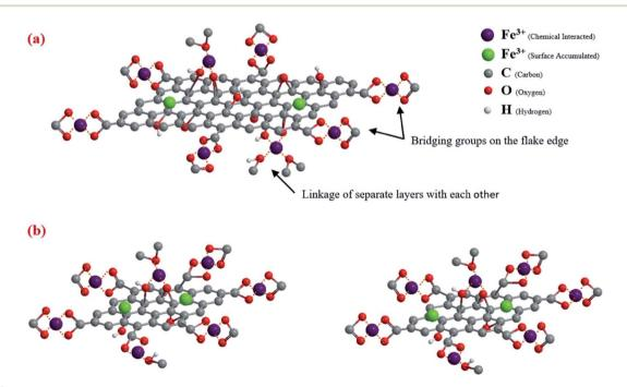
Fig. 14 Fe<sup>3+</sup> ions adsorption at GO aerogel with (a) larger flakes size (b) smaller flakes size, adapted with permission from ref. 50, copyright, Elsevier, 2019.
