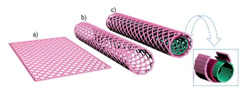
Fig. 9 Structure representations of (a) ideal graphene sheet, (b) SWCNT, and (c) MWCNTs
