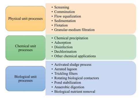
Fig. 1 Wastewater treatment unit operations and processes.
