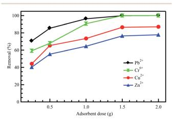
Fig. 3 Effect of adsorbent dose on the adsorption of diverse metal ions onto palm kernel shell, reproduced with permission from ref. 43, copyright, Nature, 2019.
