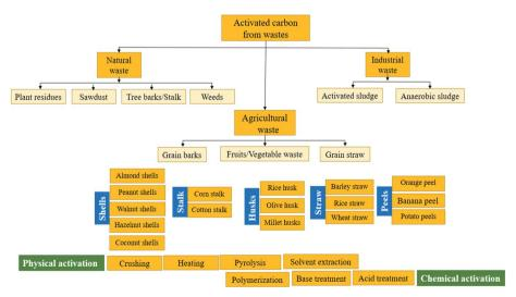
Fig. 7 Different sources and methods used for the extraction of AC
