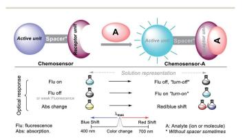
Fig. 6 Conventional configuration and optical response of a chemosensor.
