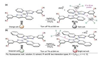
Fig. 32 Pt(II) metallomesogens for Hg<sup>2+</sup> sensing (a) 93 and (b) 94
