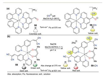
Fig. 21 Probes for CN<sup>-</sup> based on iridium complexes (a) 58 and (b) 59.
