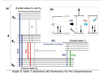
Fig. 4 (a) Jablonski diagram and (b) photophysical process.
