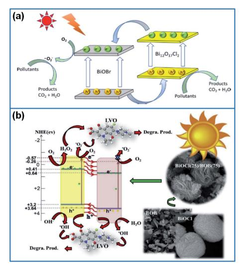
Fig. 8 (a) Schematic illustration for the transport and separation of the photo-induced electron-hole pairs and the degradation mechanism of BiOBr/Bi $_{12}O_{17}Cl_2$  composite. Sopyright 2020 Elsevier. (b) Degradation mechanism for removal of levofloxacin by using 3D flower-like BiOCl(25)/BOB(75) heterojunction photocatalysts. Copyright 2020 Elsevier.
