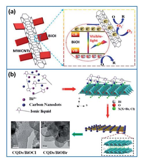
Fig. 5 (a) Photocatalytic mechanism of MWCNTs/BiOI photocatalyst.<sup>102</sup> (b) Schematic illustration of the preparation of CQDs/BiOX hybrid nanosheets and the microstructure by TEM.<sup>105</sup> Copyright 2016 Elsevier.
