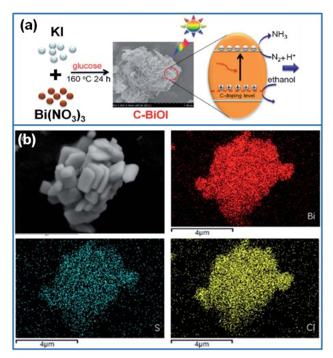
Fig. 3 (a) Preparation of C-BiOI photocatalysts by using glucose as carbon sources for degradation of organic pollutants.<sup>60</sup> Copyright 2019 Elsevier. (b) The microstructure of BiOCl-S and its element mapping.<sup>63</sup> Copyright 2018 Elsevier.
