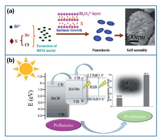
Fig. 7 (a) Schematic illustration for fabricating BiOCl/BiOBr microsphere. <sup>127</sup> Copyright 2018 Elsevier. (b) Schematic illustration of the charge transfer and separation of BiOBr/BiOF heterojunction. <sup>130</sup> Copyright 2017 Elsevier.
