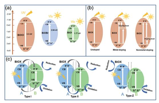
Fig. 1 The band gap structure of BiOCl, BiOBr and BiOl (a), the effect of heteroatom doping of BiOX (b) and construction of different types of BiOX heterojunctions (c).
