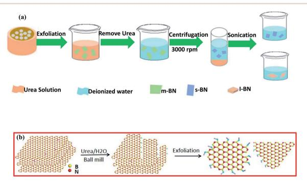
Fig. 7 (a) A flow chart showing the synthesis of small-layer BN and large-layer BN and (b) a schematic illustration of the exfoliation process using a ball-milling technique. 121
