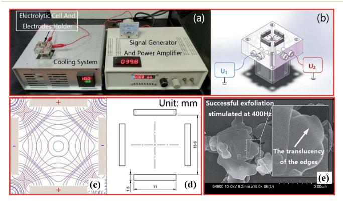
Fig. 13 (a) The assembly of the electrical stimulation system. (b) The quadrupole electrolytic cell ( $U_1$  and  $U_2$  are differential amplification voltages). (c) The rectangular quadrupole electric field (the red lines represent potential lines, and the blue lines represent field intensity lines). (d) The sizes and positions of the orthogonal titanium electrodes. (e) An SEM image of h-BN exfoliated at the optimal frequency of 400 Hz. 132
