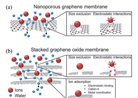
Fig. 20 Water purification via ion filtering using nanoporous graphene (a) and stacked graphene oxide (b). Reprinted with permission.<sup>33</sup> Copyright 2015, Royal Society of Chemistry.
