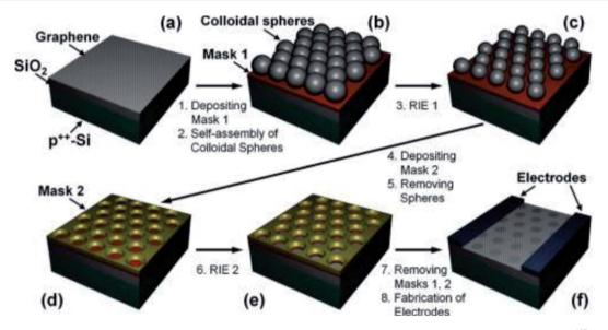
Fig. 17 Schematic of the nanomesh fabrication process using colloidal microspheres and RIE. Reprinted with permission.<sup>107</sup> Copyright 2010, American Chemical Society.
