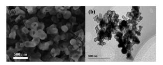
Fig. 9 (a) SEM and (b) TEM of ZnSe/MoSe<sub>2</sub>@C showing a well-defined polyhedral structure. Reproduced from ref. 83 with permission from Royal Society of Chemistry, Copyright 2019
