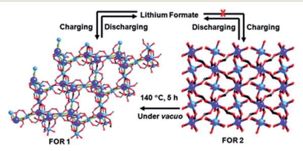
Fig. 11 Mechanism involving the formation of lithium formate (FOR) structures during charging and discharging cycles. Reproduced from ref. 158 with permission from Royal Society of Chemistry, Copyright 2010.
