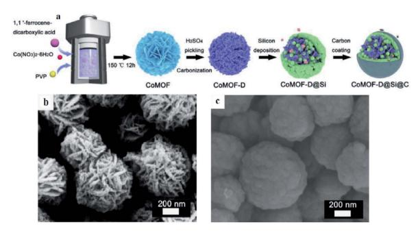
Fig. 10 (a) Schematic illustration of the synthesis of a CoMOF-D@Si@C composite; SEM images of (b) CoMOF and (c) CoMOF-D@Si@C composites. Reproduced from ref. 84 with permission from Elsevier, Copyright 2021.
