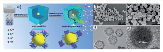
Fig. 7 (a) Scheme of preparation of a hollow Au@Zn/Ni-MOF-2 core—shell nanoreactor, (b and c) SEM and (d and e) TEM of hollow Au@Zn/Ni-MOF-2 core—shell nanocubes. Reproduced from ref. 81 with permission from American Chemical Society, Copyright 2021.
