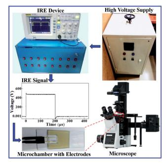
Fig. 1 The experimental set-up for the electroporation technique.
