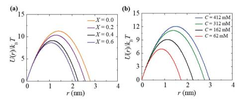
Fig. 9 The prepore free energy profiles for different values of (a) X with C=162 mM and (b) C with X=0.40 at  $\sigma=7.5$  mN m $^{-1}$ . U(r) was calculated according to eqn (8) using  $\Gamma=10.5$  pN and  $\omega=0.49$ .
