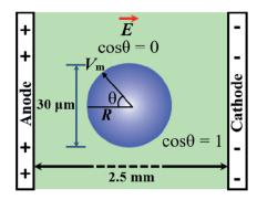
Fig. 2 The experimental design of the IRE technique for pore formation in GUVs. The electric field induces the modification of the transmembrane potential of the GUV.  $\theta$  is the angle between the radius of the GUV (R) (from the GUV center to the evaluation point) and the electric field.
