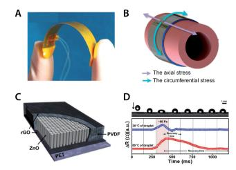
Fig. 3 (A) Self-powered PVDF thin film based blood pressure sensor. (B) Circumferential and axial stress on aorta wall. Reproduced from ref. 166, with permission from Elsevier. (C) Schematic design of ZnO/PVDF based pressure and temperature sensor. (D) Top graph: mechanical impact of droplet onto sensor with unknown temperature. Bottom graph: corresponding resistance and recovery time upon impact of different temperature droplets. Reproduced from ref. 173, with permission from Springer Nature.
