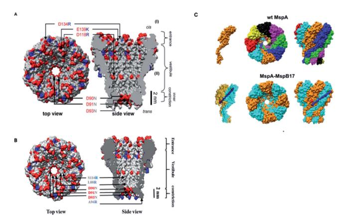
Fig. 3 MspA mutants. Genetically engineered mutants of MspA nanopores (A) M1MspA and M2MspA,<sup>99</sup> (B) M3MspA and (C) stoichiometric mutant of MspA, MspA–MspB17.<sup>100</sup> Figures do not need permission from the references.
