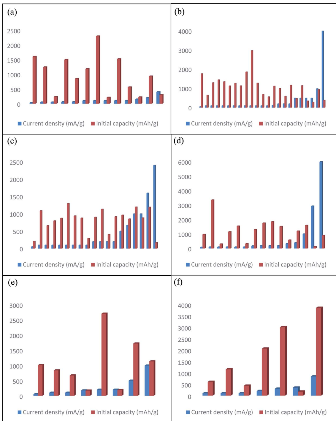
Fig. 8 Highest initial capacity at the certain current density of (a) CNT, 24–26,30,31,33,36,39,40,42–44,48 (b) CNFs, 52,55–60,62–75,77,78 (c) graphene, 85–87,90–102,104,105,107 (d) CFT, 111,113–120,122,123,125,126,129,130,134–136,138,142–145 (e) carbon coating/foam, 134–136,138,142–145 and (f) metals-supported 178,179,181,184,190,192 flexible electrodes.
