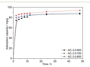
$\begin{tabular}{lll} Fig. & Adsorption & capacities & of & ACs & with & various & activation \\ temperatures. & \\ \end{tabular}$
