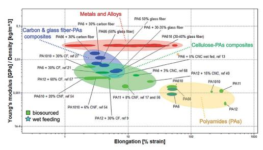
Fig. 4 Ashby plot of specific Young's modulus as a function of the elongation for neat PAs and their different fibres composites compared with main engineering materials in use.
