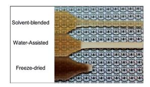
Fig. 5 Differences in the thermal degradation of the cellulose component in PA6/CNC composites processed with three different compounding approaches, as indicated by the darkening of the specimens.<sup>60</sup>
