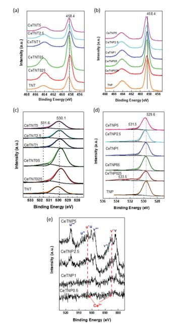
Fig. 3 XPS core level spectra: (a and b) Ti 2p signals of CeTNTx and CeTNP, respectively; (c and d) O 1s signals of CeTNTx and CeTNP, respectively; and (e) Ce 3d spectra of CeTNP samples.
