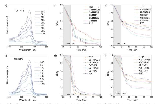
Fig. 4 (a and b) UV-Visible spectra recorded at different times, from 30 min under dark conditions (30D) to 120 min under UV light irradiation (120L), for the two 5.0 wt%  $CeO_2$ - $TiO_2$  nanostructures: (a) CeTNT5 sample and (b) CeTNP5 sample. (c-f) MB photodegradation test in aqueous solution: CeTNTx (c) under UV light irradiation and (e) under simulated solar light; and  $CeTNP_x$  (d) under UV light irradiation and (f) under simulated solar light.
