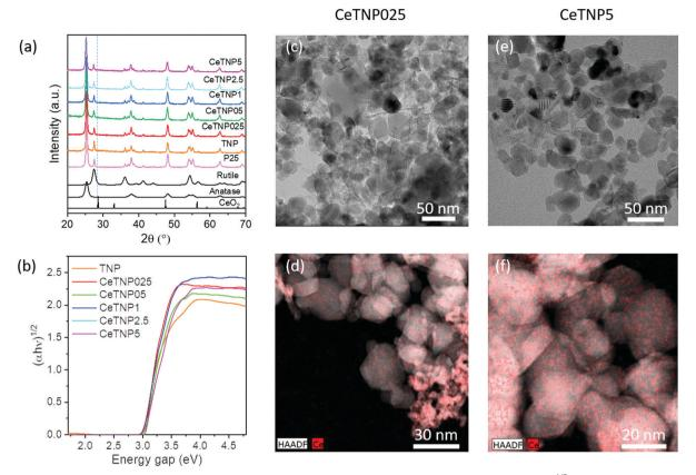
Fig. 2 Undoped and Ce-doped TNP series. (a) XRD patterns, including benchmarking anatase, rutile and P25. (b)  $(\alpha h \nu)^{1/2}$  vs. photoenergy (eV) plot. TEM/ HAADF images for samples CeTNP025 (c and d) and CeTNP5 (e and f). (d) and (f) show the EDS maps for Ce overlapping the STEM images.
