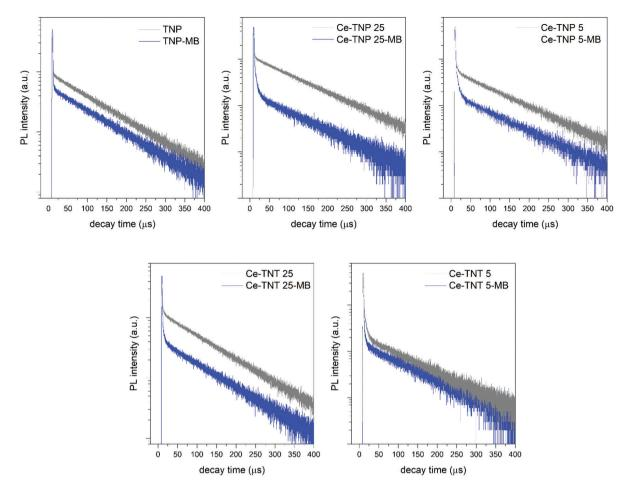
TRPL decay spectra for selected samples of the two TNP and TNT series.  $\lambda_{ex}$  = 250 nm;  $\lambda_{em}$  = 400 nm.
