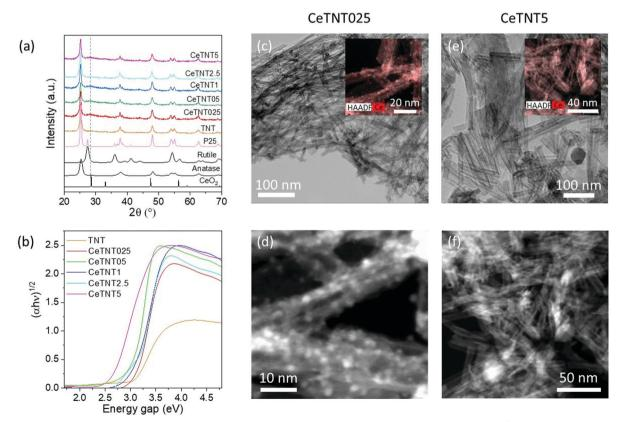
Fig. 1 Undoped and Ce-doped TNT series. (a) XRD patterns, including benchmarking anatase, rutile and P25. (b)  $(\alpha h \nu)^{1/2}$  vs. photoenergy (eV) plot. TEM/ HAADF images for samples CeTNT025 (c and d) and CeTNT5 (e and f). The insets in (c) and (e) show the EDS maps for Ce overlapping the STEM images.
