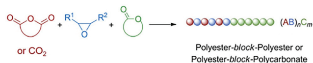
Fig. 14 One-shot switchable copolymerization of epoxide, anhydride ( \text{CO}_2 ) and lactone using a dizinc catalyst, obtaining polyester (polycarbonate)- b -polyester block copolymers by sequential ROCOP of epoxides/anhydrides ( \text{CO}_2 ) and ROP of lactones.
