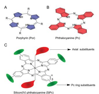
Fig. 1 Chemical structures of (A) porphyrin (Por), (B) phthalocyanine (Pc) and (C) silicon( $\bowtie$ ) phthalocyanine (SiPc). R denotes various alkyl or aryl groups. The axial substituents are highlighted as red teardrops. The phthalocyanine ring ( $\alpha$ ) and ( $\beta$ ) substituents are highlighted as green ovals.
