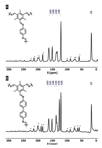
Fig. 2 Solid-state NMR spectra of Me<sub>3</sub>TFB-PA (A) and Me<sub>3</sub>TFB-BD (B). The signal at 162 ppm can be assigned to the carbon of an imine-bound nitrogen, indicating the formation of imine bonds. Spinning side bands, here indicated with an asterisk, were determined by comparing different MAS frequencies
