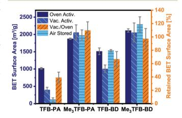
Fig. 3 BET surface areas with different activation methods (oven-dried and vacuum-dried) and after four weeks stored on the bench. The retained BET surface area gives the ratio how much  $S_{\text{BET}}$  has been left after vacuum drying. The errors result from the analyses of three
