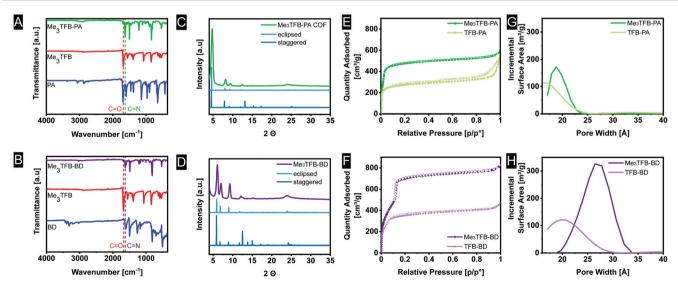
Fig. 1 Characteristics of Me<sub>3</sub>TFB-PA (top) and Me<sub>3</sub>TFB-BD (bottom): FT-IR spectra of COFs and starting materials (A and B), PXRD spectra including simulated PXRD patterns (C and D), nitrogen sorption isotherms including their non-methylated references (E and F) and pore size distributions (G and H).
