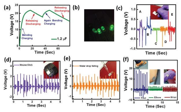
Fig. 3 (a) Charging-discharging behavior of a capacitor of 1.2 µF using the PENG device, (b) glowing of four green commercial LEDs (I<sub>power</sub> = 110 mW (max)). The output voltage from the PENG device due to (c) writing on paper, (d) clicking of a computer mouse, (e) falling water drops and (f) different human body movements and the images are shown in insets.
