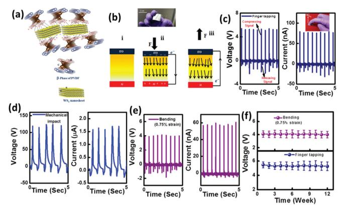
Fig. 2 Schematic mechanisms of (a) interactions between WS<sub>2</sub> and PVDF and (b) operation of a piezo-electric nanogenerator and the device image is shown in the inset. Open-circuit output voltage and current from the PVDF-WS2 PENG for 0.187% filler loading for repeated (c) finger tapping, (d) mechanical impact (~105 kPa) and (e) bend/release action, (f) long-term stability performance of the PVDF-WS2 PENG in laboratory atmosphere for 12 weeks on repeated mechanical tapping and bending
