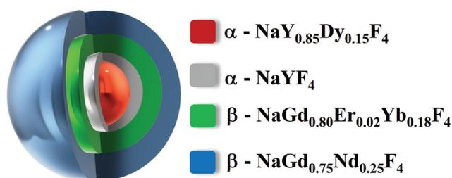
Fig. 1 Schematic illustration of the core@multi-shell nanoarchitecture.
