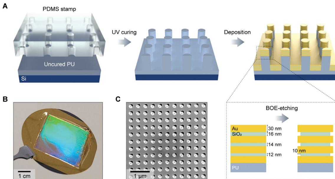
**Fig. 1** Fabrication of 3D nanolaminate plasmonic crystals (NLPC) as a SERS substrate for dopamine (DA) sensing. (A) Schematic illustration of the fabrication process for a 3D NLPC SERS substrate. (B) Photographic and (C) top-view SEM images of a 3D NLPC SERS substrate.
