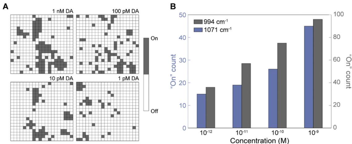
**Fig. 6** Digital SERS sensing for the quantitative determination of DA. (A) Digital mapping images with different DA concentrations converted from those in Fig. 5A. (B) Histogram of the total number of "On" spectra using two main peaks for 3-MPBA at 994 and 1071 cm<sup>-1</sup> (the yellow lines in Fig. 5B).
