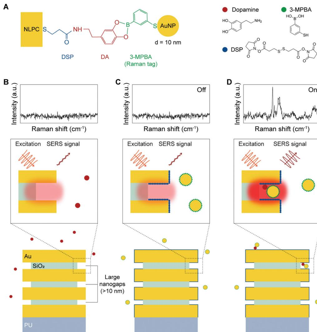
**Fig. 3** Digital SERS sensing platform using the 3D NLPC-based dual-recognition structure coupled with AuNPs for quantitative DA detection. (A) Molecular sensing scheme for the specific targeting of DA via a 3D NLPC-based dual-recognition structure. (B) Label-free SERS sensing. DA-specific dual-recognition structure, producing (C) an "Off" state in the absence of DA and (D) an "On" state in the presence of DA.
