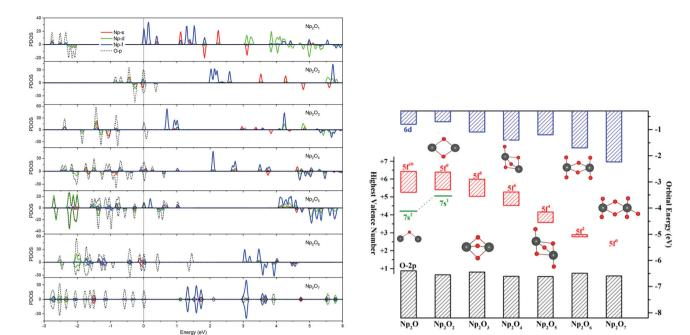
Fig. 2 The formal oxidation state of Np along with the series together with the corresponding values for the HOMO-LUMO gaps of Np<sub>2</sub>O<sub>x</sub> (x = 1 to 7).
