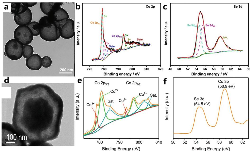
Fig. 20 (a) TEM image of CoSe<sub>2</sub>-30. (b) Co 2p and (c) Se 3d XPS spectra of CoSe<sub>2</sub>-30.<sup>49</sup> Copyright © 2019 Elsevier B.V. All rights reserved. (d) HR-TEM image of Y-S Ni-Co-Se. XPS spectra of the (e) Co 2p and (f) Se 3d regions.<sup>164</sup> Copyright © 2018, American Chemical Society.
