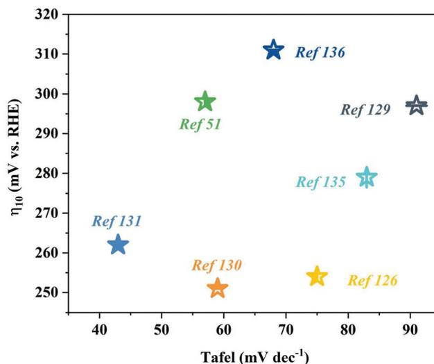
Fig. 15 OER activity comparison graph showing the Tafel slope versus overpotential at a current density of 10 mA cm<sup>-2</sup> for different catalysts.
