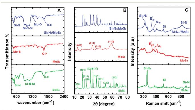
Fig. 1 (A) FTIR spectra, (B) XRD patterns, and (C) Raman spectra of Si<sub>3</sub>N<sub>4</sub>, MoS<sub>2</sub> and the Si<sub>3</sub>N<sub>4</sub>/MoS<sub>2</sub> composite.
