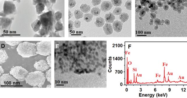
Fig. 3 TEM images of (A) Fe<sub>3</sub>O<sub>4</sub> NPs and (B and C) MMSNs, (D) SEM image of MMSNs@AuNPs, (E) HRTEM image of MMSNs@AuNPs, and (F) EDX spectra of MMSNs@AuNPs.
