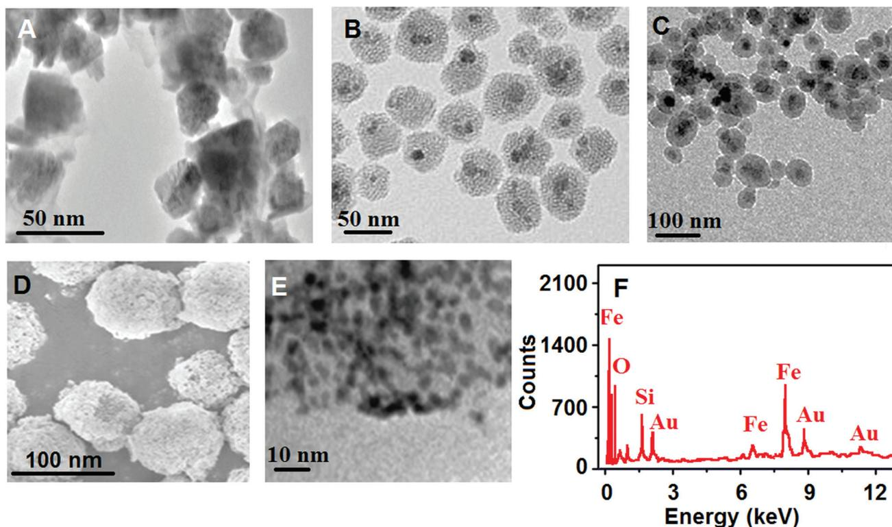
Fig. 3 TEM images of (A)  $\text{Fe}_3\text{O}_4$  NPs and (B and C) MMSNs, (D) SEM image of MMSNs@AuNPs, (E) HRTEM image of MMSNs@AuNPs, and (F) EDX spectra of MMSNs@AuNPs.
