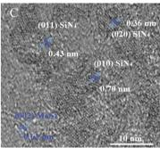
Fig. 2 TEM images (A-C) of the Si<sub>3</sub>N<sub>4</sub>/MoS<sub>2</sub> composite.
