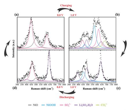
Fig. 4 Raman spectra of the electrode/electrolyte interface under cyclic voltammetry at a scan rate of 0.15 mV  $\rm s^{-1}$  from (a) 0 to (b) 1 V during charge and from (c) 1 V to (d) 0 V during discharge. Spectra intensities are normalized from 0 to 1 in the 300 to 800 cm<sup>-1</sup>. Working electrodes were housed in a symmetrical El Cell filled with 80 µL of a 1 M Li<sub>2</sub>SO<sub>4</sub> aqueous solution.
