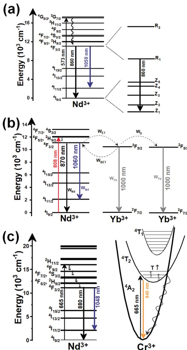
Fig. 21 Mechanisms of generation of the emission lines of: (a) single-doped  $\text{Nd}^{3+}$  luminescent thermometers excited at 573 nm, (b) dual emitting center  $\text{Nd}^{3+}/\text{Yb}^{3+}$  luminescent thermometers excited at 808 nm, and (c) dual emitting center  $\text{Nd}^{3+}/\text{Cr}^{3+}$  luminescent thermometers excited at 665 nm, operating simultaneously in the I- and II-BWs.
