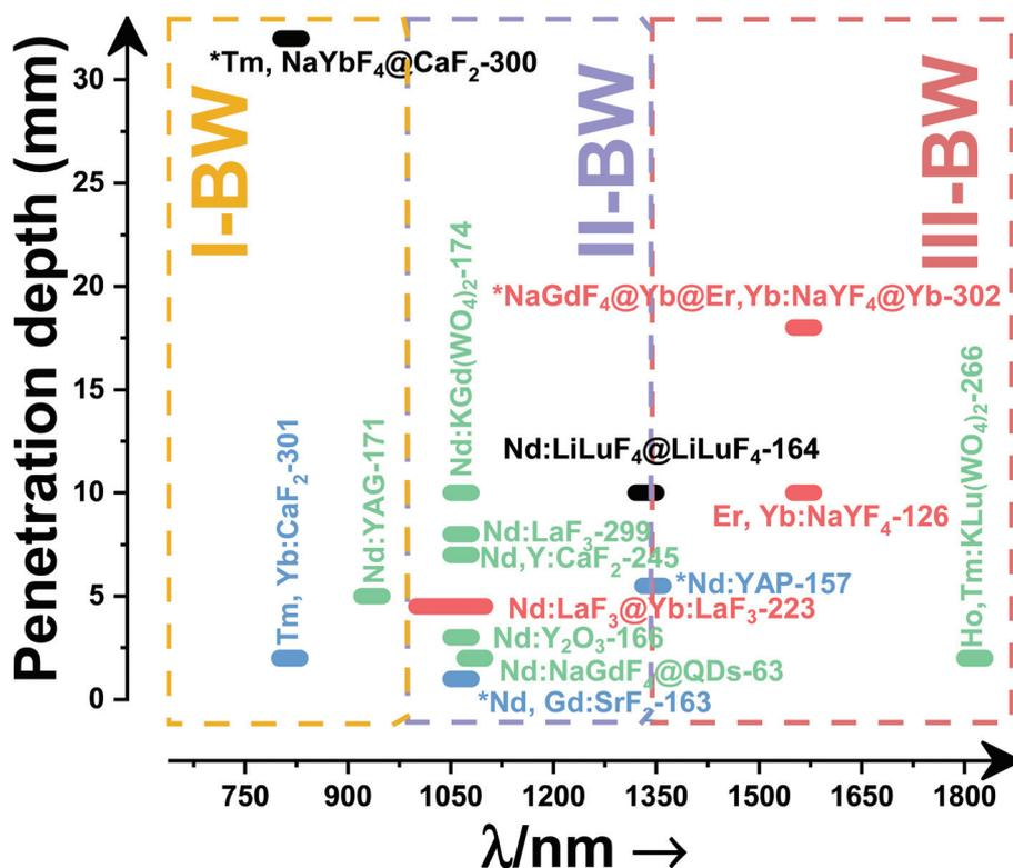
Fig. 57 Penetration depth in the BWs spectral regions reported for Ln<sup>3+</sup>-doped luminescent nanomaterials. The intervals represent the operating wavelength regimes for the corresponding nanothermometer, whereas the asterisk indicates only one reported wavelength. The black, blue, red and green colors stand for the different types of biological medium: black = pork tissue, blue = phantom tissue, red = mice and green = chicken tissue. The numbers are the corresponding references.
