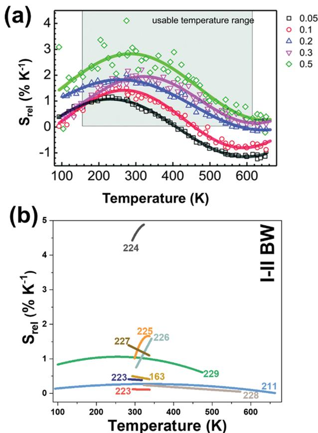
Fig. 22 (a)  $S_{\text{rel}}$  of  $\text{Nd}^{3+}$ - and  $\text{Yb}^{3+}$ -doped  $\text{LiLaP}_4\text{O}_{12}$  as a function of  $\text{Yb}^{3+}$  concentration. Reprinted with permission from ref. 201. Copyright 2015, the Owner Societies. (b) Temperature dependence of  $S_{\text{rel}}$  of lanthanide-doped luminescent thermometers operating in the I-BW and II-BWs, simultaneously. The numbers indicate the corresponding references for each thermometer.
