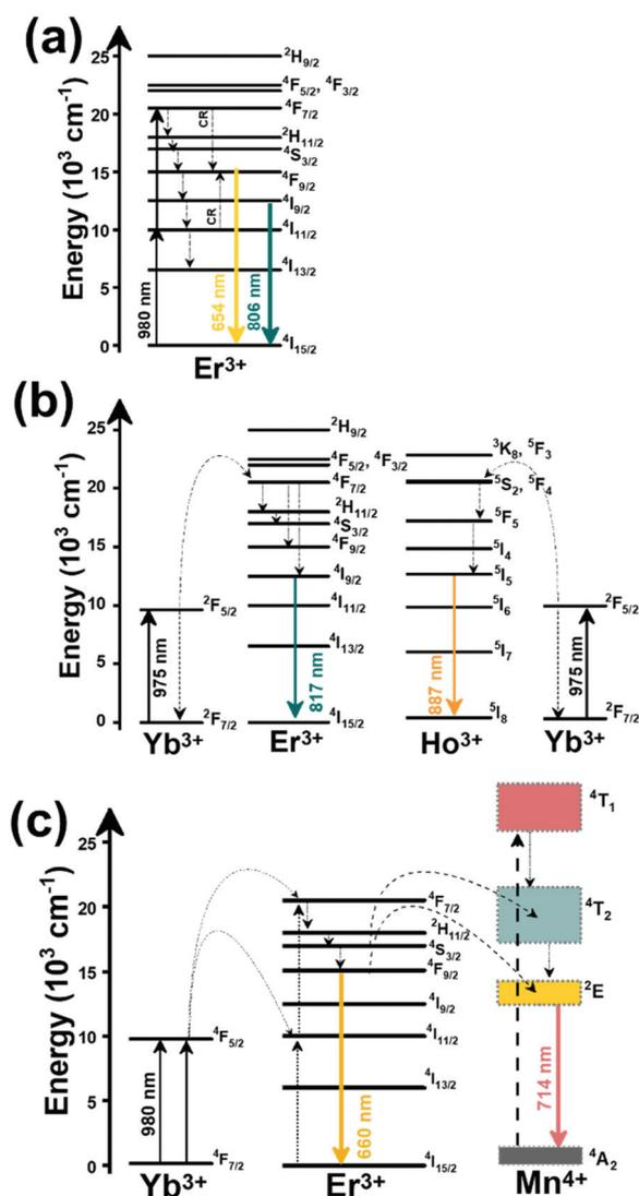
Fig. 18 Mechanisms of generation of the emission lines located in the I-BW of: (a) Er<sup>3+</sup>, (b) Er<sup>3+</sup>/Ho<sup>3+</sup>/Yb<sup>3+</sup>, and (c) Er<sup>3+</sup>/Mn<sup>4+</sup>/Yb<sup>3+</sup> doped materials.
