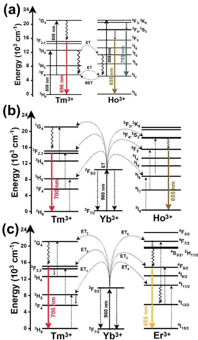
Fig. 9 Mechanisms of generation of the emission lines for: (a)  $\text{Tm}^{3+}$ ,  $\text{Ho}^{3+}$ -doped  $\text{KLu}(\text{WO}_4)_2$  nanocrystals after excitation at 808 nm, (b)  $\text{Tm}^{3+}$ ,  $\text{Ho}^{3+}$ ,  $\text{Yb}^{3+}$ -doped  $\text{YPO}_4$  or  $\text{Gd}_2(\text{WO}_4)_3$  nanoparticles after excitation at 980 nm, and (c)  $\text{Tm}^{3+}$ ,  $\text{Er}^{3+}$ ,  $\text{Yb}^{3+}$ : $\text{YF}_3$  nanoparticles embedded in a glass ceramic after excitation at 980 nm.
