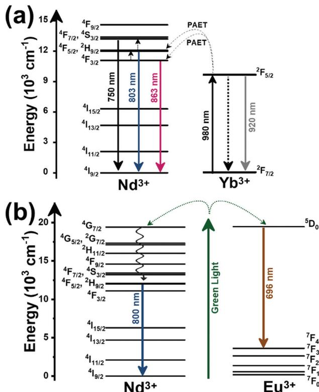
Fig. 13 Mechanisms of generation of the emission bands of nanoparticles codoped with  $\text{Nd}^{3+}$  and: (a)  $\text{Yb}^{3+}$  after 980 nm excitation, and (b)  $\text{Eu}^{3+}$  after excitation in the green range.
