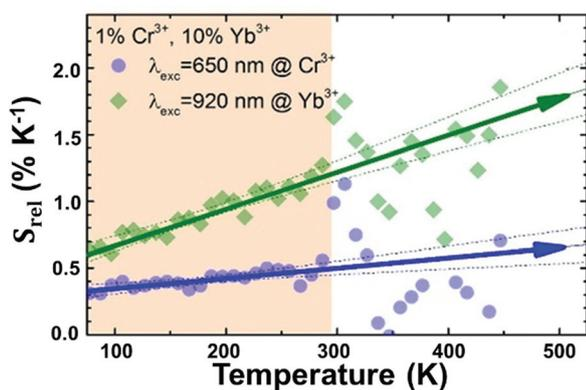
Fig. 25  $S_{\text{rel}}$  of codoped  $\text{Cr}^{3+}, \text{Yb}^{3+}:\text{LiLaP}_4\text{O}_{12}$  nanoparticles operating simultaneously in the I- and II-BWs, as a function of the excitation wavelength. Reprinted with permission from ref. 229. Copyright 2016, Elsevier.
