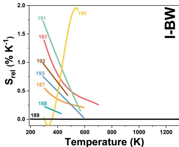
Fig. 19 Temperature dependence of  $S_{\text{rel}}$  of  $\text{Er}^{3+}$ -doped luminescent thermometers, operating in the I-BW. The numbers represent the corresponding references for each  $\text{Er}^{3+}$ -based thermometer.
