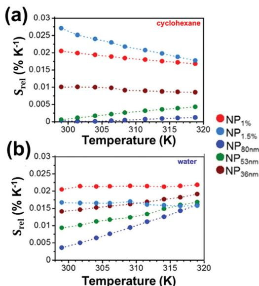
**Fig. 35**  $S_{\text{rel}}$  of  $\text{Er}^{3+}, \text{Ho}^{3+}, \text{Yb}^{3+}:\text{NaYF}_4$  nanocrystals as a function of dispersing agents: (a) cyclohexane and (b) distilled water. Also the effect of the  $\text{Ho}^{3+}$  concentration (1.5 mol% and 3 mol%) and the size of the nanocrystals (36 nm, 53 nm and 83 nm) can be observed. Adapted with permission from ref. 252. Copyright 2016, Elsevier.
