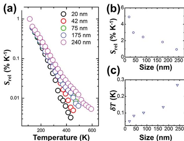
Fig. 23 The effect of the size of  $\text{Nd}^{3+}, \text{Cr}^{3+}:\text{LiLaP}_4\text{O}_{12}$  nanoparticles on: (a) the intensity ratio between the emissions lines of  $\text{Cr}^{3+}$  and  $\text{Nd}^{3+}$  at 810 nm and 1048 nm, respectively, (b)  $S_{\text{rel}}$ , and (c)  $\delta T$ . Reprinted with permission from ref. 232. Copyright 2016, Elsevier.
