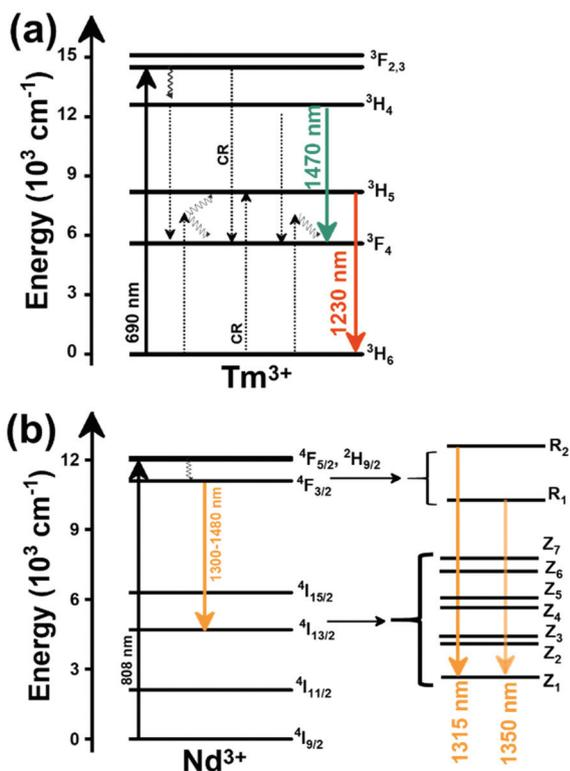
Fig. 38 Mechanism of the generation of the emission lines on: (a)  $\text{Tm}^{3+}$ -doped  $\text{LaF}_3$  nanocrystals, and (b)  $\text{Nd}^{3+}:\text{Gd}_2\text{O}_3$  nanospheres, operating in the II-BW and III-BW regions simultaneously.
