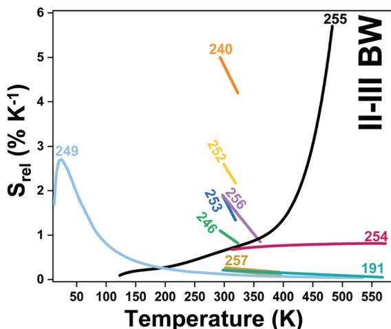
Fig. 33 Temperature dependence of  $S_{\text{rel}}$  of all nanothermometers operating simultaneously in the II- and III-BW regions. Numbers represent the corresponding literature references for each thermometer.
