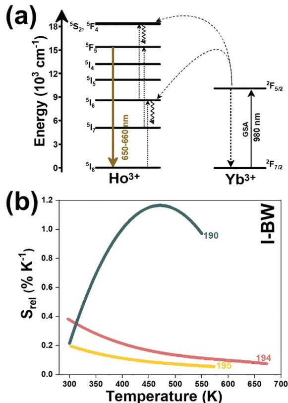
Fig. 20 (a) Mechanism of generation of the emission lines of  $\text{Ho}^{3+}/\text{Yb}^{3+}$ -doped luminescent thermometers. (b) Temperature dependence of  $S_{\text{rel}}$  of  $\text{Ho}^{3+}$ -doped luminescent thermometers operating in the I-BW. The numbers represent the references for each  $\text{Ho}^{3+}$ -based thermometer.
