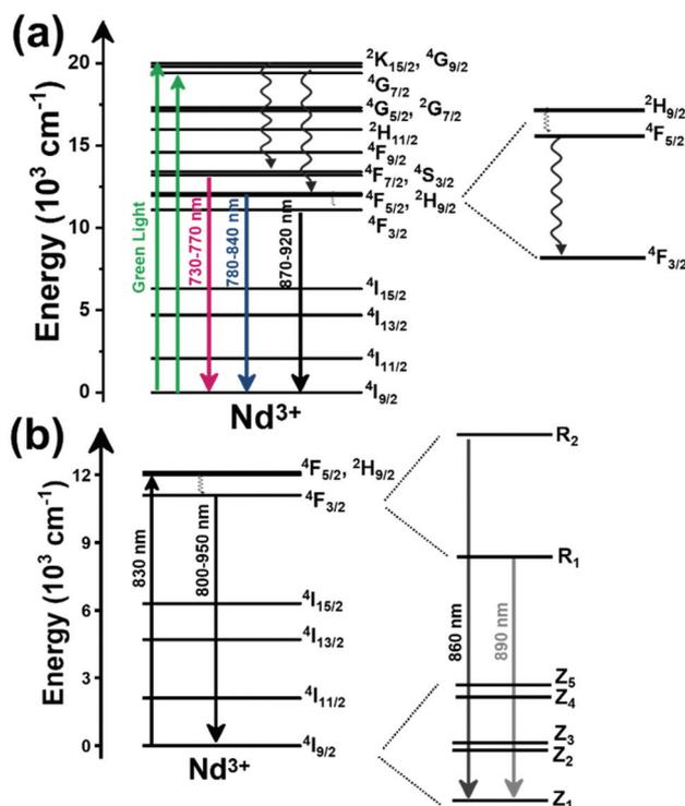
Fig. 11 Mechanisms of generation of the emission bands in single  $Nd^{3+}$ -doped nanoparticles after being excited with: (a) a green light source (the magnification detail depicts the thermally coupled  ${}^4F_{5/2}$  and  ${}^4F_{3/2}$  levels), and (b) a near infrared light source.
