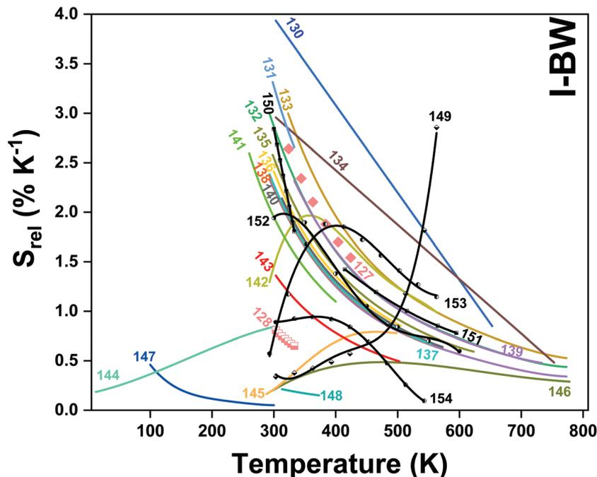
Fig. 7 Temperature dependence of  $S_{\text{rel}}$  of  $\text{Tm}^{3+}$ -doped luminescent thermometers, operating in the I-BW. In symbols only, in solid lines and in solid lines with symbols, single  $\text{Tm}^{3+}$ ,  $\text{Tm}^{3+}/\text{Yb}^{3+}$  and  $\text{Tm}^{3+}/\text{Ln}^{3+}$  based thermometers, respectively. The numbers represent the corresponding references for each  $\text{Tm}^{3+}$ -based thermometer.
