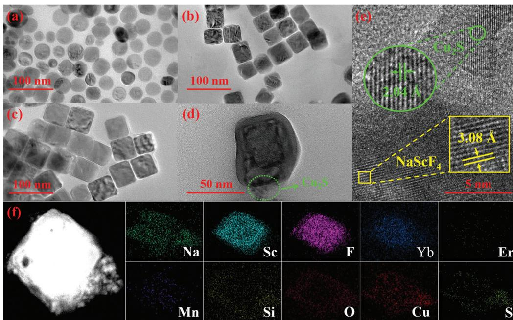
Fig. 2 TEM images of (a) NYEM, (b) NYEM@NaScF<sub>4</sub>, (c) NYEM@NaScF<sub>4</sub>@SiO<sub>2</sub> and (d) NYEM@NaScF<sub>4</sub>@SiO<sub>2</sub>@Cu<sub>2</sub>S. (e) A HR-TEM image and (f) element mapping images of NYEM@NaScF<sub>4</sub>@SiO<sub>2</sub>@Cu<sub>2</sub>S.
