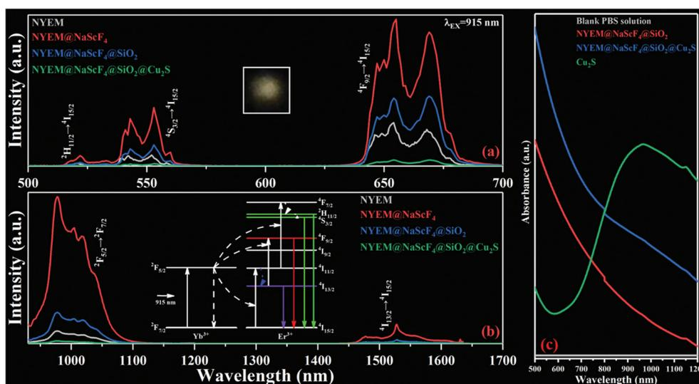
Fig. 3 (a) UC spectra and (b) NIR spectra of the prepared samples. (c) Absorption spectra of NYEM@NaScF<sub>4</sub>@SiO<sub>2</sub>, NYEM@NaScF<sub>4</sub>@SiO<sub>2</sub>@Cu<sub>2</sub>S and Cu<sub>2</sub>S dispersed in PBS solution as well as the blank PBS solution. The inset in (a) is the digital photo of NYEM@NaScF<sub>4</sub>@SiO<sub>2</sub>@Cu<sub>2</sub>S excited by 915 nm wavelength. The inset in (b) is the ET processes between Yb<sup>3+</sup> and Er<sup>3+</sup>.
