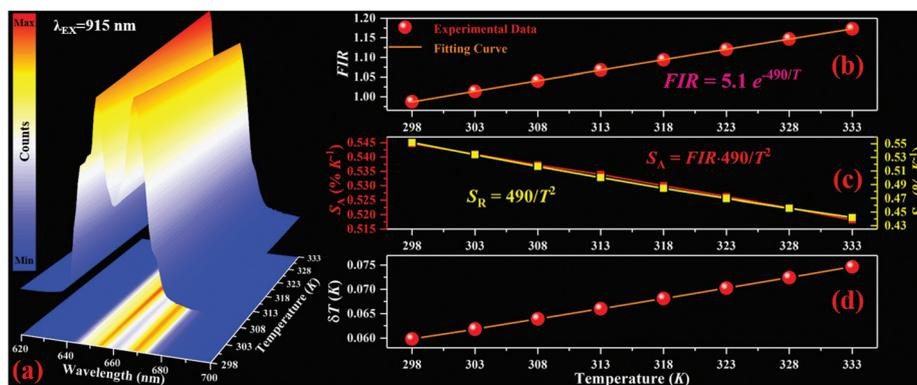
Fig. 4 (a) Red UC emission normalized at 669 nm, (b) FIR, (c) absolute sensitivity  $S_A$  and relative sensitivity  $S_R$  and (d) temperature resolution  $\delta T_G$  as a function of temperature in  $\text{NYEM@NaScF}_4@\text{SiO}_2@\text{Cu}_2\text{S}$ .
