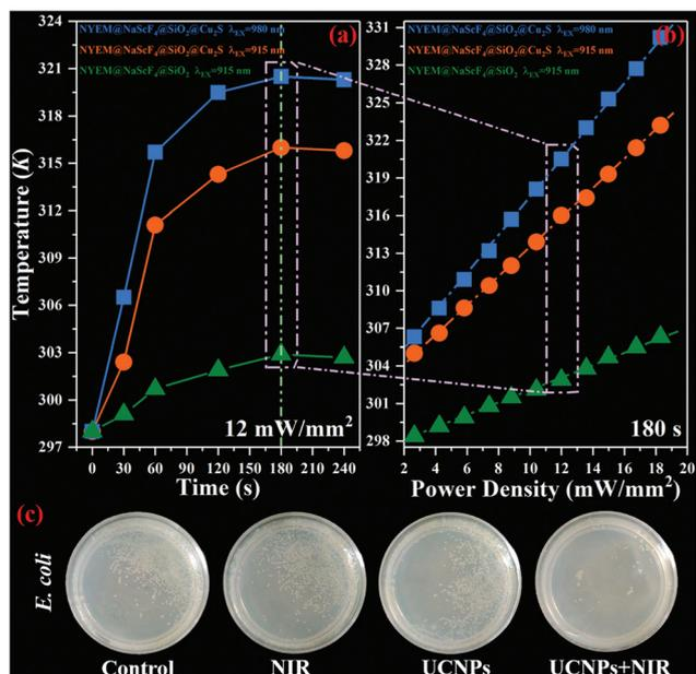
Fig. 5 The photothermal conversion effect of NYEM@NaScF<sub>4</sub>@SiO<sub>2</sub> and NYEM@NaScF<sub>4</sub>@SiO<sub>2</sub>@Cu<sub>2</sub>S dispersed in PBS solution versus (a) excitation time and (b) power density. (c) Digital photos of *E. coli* incubated within various conditions.
