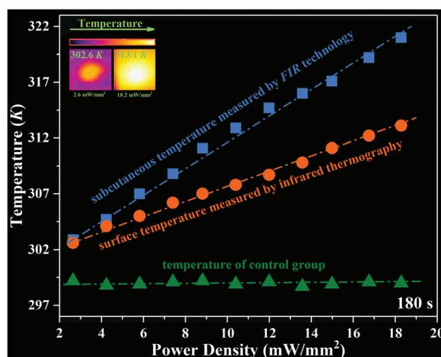
Fig. 6 The subcutaneous temperature and surface temperature of chicken tissue injected with NYEM@NaScF<sub>4</sub>@SiO<sub>2</sub>@Cu<sub>2</sub>S NPs versus the power density of the 915 nm laser and chicken tissue without NPs is used as the control group.
