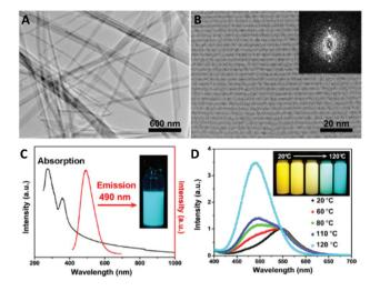
Fig. 22 (A) TEM image of the ribbons from CuNCs self-assembly. (B) HRTEM image of the ribbons. Inset: Fourier transform image. (C) Steadystate absorption (black) and emission (red) spectra of the ribbons in chloroform. Inset: The fluorescent image with 365 nm excitation. (D) Spectra of CuNCs assemblies respectively prepared at 20, 60, 80, 110, and 120 °C. Inset: Sample excited at 365 nm at different temperatures. Reprinted with permission from ref. 139. Copyright 2015 American Chemical Society.
