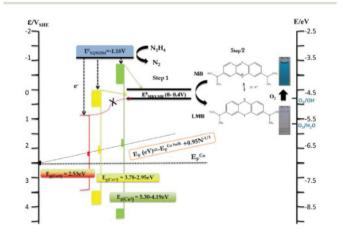
Fig. 36 Schematic energy diagram showing the catalytic activity of different CuNCs used for MB reduction by  $N_2H_4$ . Reprinted with permission from ref. 423. Copyright 2012 American Chemical Society.
