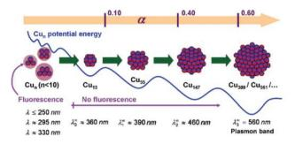
Fig. 5 Schematic representation of copper nanocluster size evolution with increasing the molar percentage (a) of NaBH<sub>4</sub>. The clusters with  $n \le 13$  are fluorescent, whereas big particles with  $n \ge 309$  show characteristic plasmon resonance band. Reprinted with permission from ref. 101. Copyright 2009 American Chemical Society.
