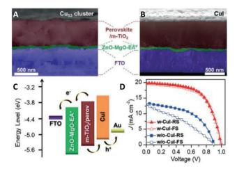
Fig. 38 Device structure and cross-sectional SEM image of (A) Cu<sub>53</sub> and (B) Cul on perovskite films. (C) Energy-level diagram of Cul-based perovskite solar cell (PSC). (D) Best J-V curves of devices with Cul (w-Cul) and without Cul (w/o-Cul). FS = forward scan, RS = reverse scan. Adapted with permission from ref. 194. Copyright 2019 Wiley-VCH Verlag GmbH &Co. KGaA, Weinheim.
