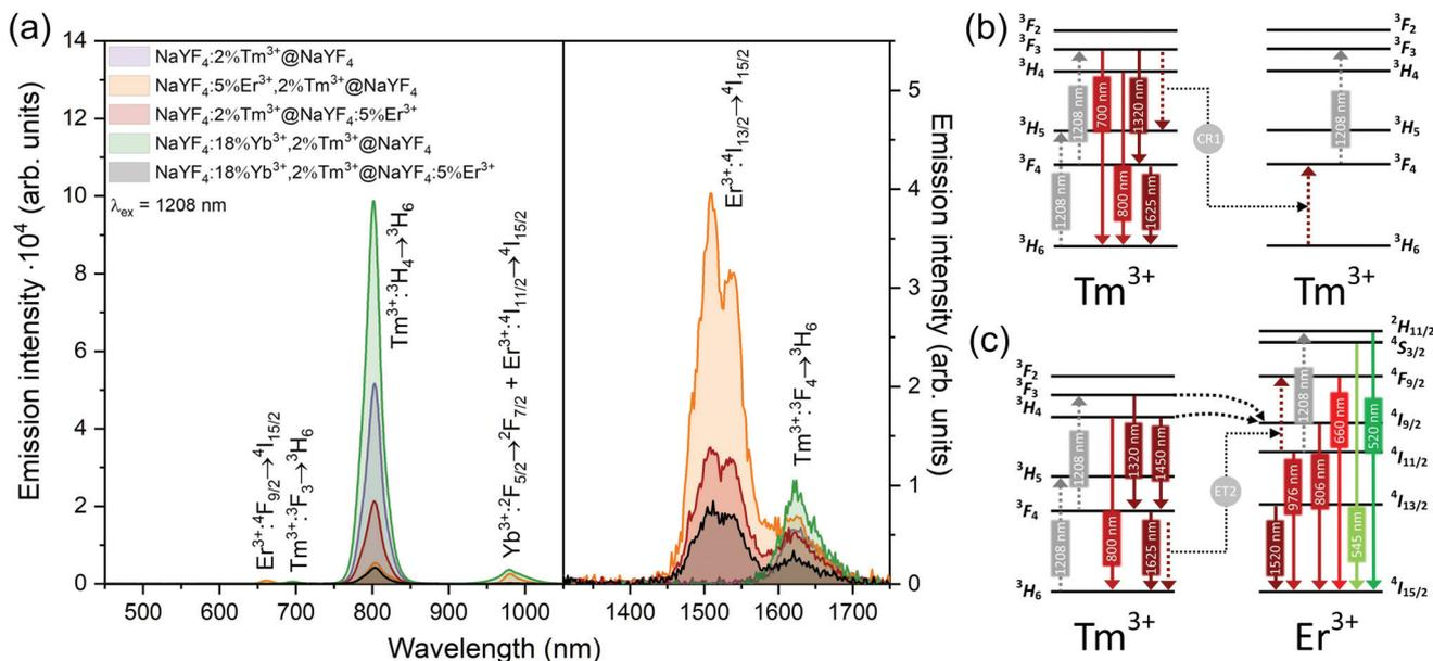
Fig. 6 (a) Emission of core@shell NPs collected under excitation by 1208 nm laser radiation ( $15 \text{ W cm}^{-2}$ ). Left spectra were measured using a CCD camera and right spectra used a NIR PMT. (b and c) Simplified UC mechanisms responsible for the observed emission of NPs doped with (b) Tm<sup>3+</sup> or (c) Er<sup>3+</sup> and Tm<sup>3+</sup> ions under 1208 nm laser excitation.
