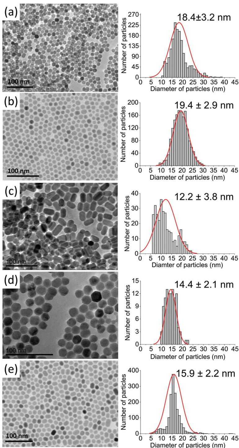
Fig. 2 TEM images recorded for (a)  $\text{NaYF}_4:2\%\text{Tm}^{3+}@NaYF_4$ , (b)  $\text{NaYF}_4:2\%\text{Tm}^{3+},5\%\text{Er}^{3+}@NaYF_4$ , (c)  $\text{NaYF}_4:2\%\text{Tm}^{3+}@NaYF_4:5\%\text{Er}^{3+}$ , (d)  $\text{NaYF}_4:18\%\text{Yb}^{3+},2\%\text{Tm}^{3+}@NaYF_4$ , and (e)  $\text{NaYF}_4:18\%\text{Yb}^{3+},2\%\text{Tm}^{3+}@NaYF_4:5\%\text{Er}^{3+}$  NPs.
