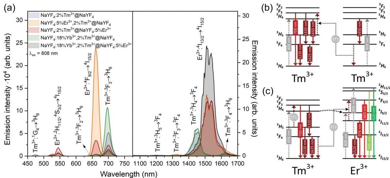
Fig. 4 (a) Emission of core@shell NPs in the Vis and NIR range under excitation by 808 nm laser radiation ( $15 \text{ W cm}^{-2}$ ). On the left, spectra were measured using a CCD camera, whereas spectra on the right used an NIR PMT (b and c) possible energy transfer schemes in NPs doped with (b)  $\text{Tm}^{3+}$  or (c)  $\text{Er}^{3+}$  and  $\text{Tm}^{3+}$  ions under 808 nm laser excitation.
