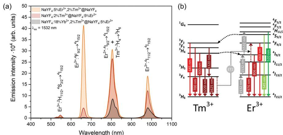
Fig. 7 (a) Emission of synthesised core@shell NPs under 1532 nm laser excitation ( $15 \text{ W cm}^{-2}$ ). (b) Possible energy transfers in NPs doped with  $\text{Er}^{3+}$  and  $\text{Tm}^{3+}$  ions under 1532 nm laser excitation.
