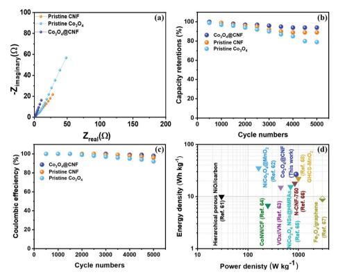
Fig. 7 Electrochemical performance of the SSC devices for the pristine Co<sub>3</sub>O<sub>4</sub> nanoparticles, pristine CNF and 1D Co<sub>3</sub>O<sub>4</sub>@CNF hybrid electrodes: (a) EIS plot, (b and c) capacity of retentions and coulombic efficiency of electrodes at 15 A g<sup>-1</sup> of current density over 5000 cycles and (d) Ragone plot.
