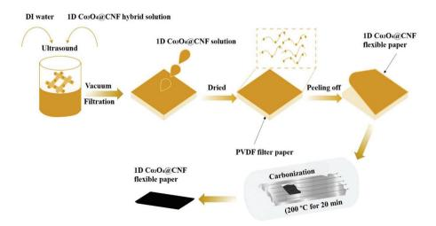
$\begin{tabular}{ll} Scheme 1 & Schematic vacuum filtration preparation of the 1D Co$_3O_4@CNF flexible paper electrode. \end{tabular}$
