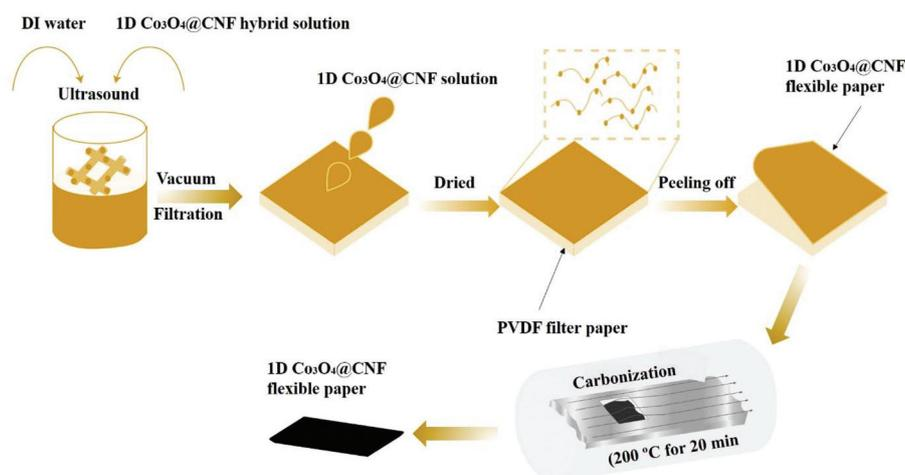
**Scheme 1** Schematic vacuum filtration preparation of the 1D Co<sub>3</sub>O<sub>4</sub>@CNF flexible paper electrode.
