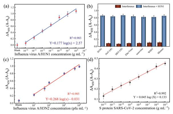
Fig. 4 (a) The calibration line for the detection of IV/A/H1N1 by TMB-NPs@PLGA based colorimetric detection in the PBS system; (b) the selectivity test in the presence of interferences. The calibration curve obtained using the clinically isolated IV/A/H3N2 (c) and recombinant spike protein of SARS-CoV-2 (d).  $A_0$  indicates the absorbance of a blank sample. The error bars represent the standard deviation of the three measurements.
