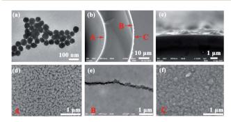
Fig. 2 (a) TEM image of AuNPs. (b and c) SEM images of the end face of the silver-coated capillary at different magnifications. (d-f) SEM images of the top view of surfaces A, B and C, which were indicated in (b).
