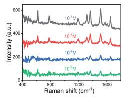
Fig. 7 Raman spectra of R6G with concentrations ranging from  $10^{-5}\,\mathrm{M}$  to  $10^{-8}\,\mathrm{M}$  detected by a portable Raman spectrometer. The output light from the Raman probe head was coupled into a multimode fiber which aligns with the capillary using a common flange optical fiber connector.
