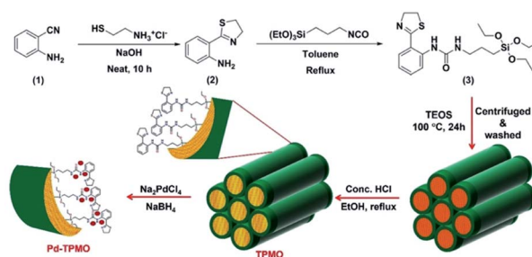
Fig. 38 Synthesis of the thiazoline-silyl precursor, thiazoline bridged periodic mesoporous organosilica (TPMO) and Pd NP entrapped TPMO (Pd-TPMO). 199 Reproduced with permission. 199 Copyright 2012, John Wiley & Sons.
