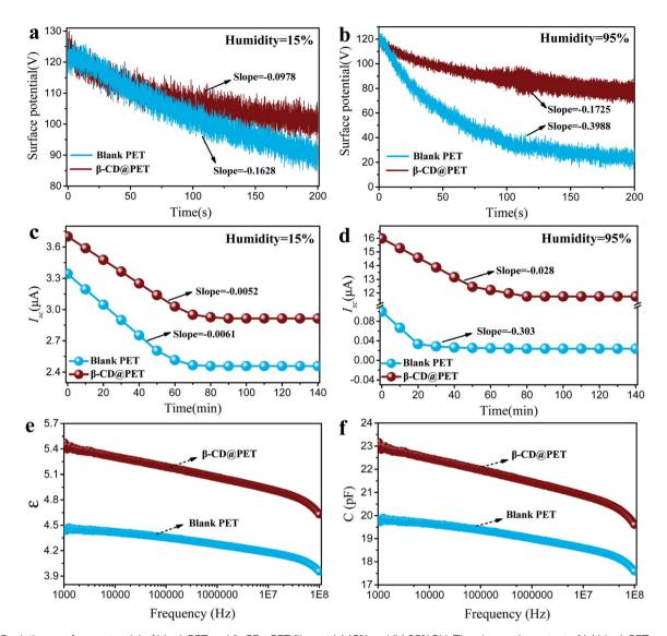
Fig. 6 Real-time surface potential of blank PET and  $\beta$ -CD@PET films at (a) 15% and (b) 95% RH. The charge decay test of (c) blank PET- and (d)  $\beta$ -CD@PET-based TENGs at 15% and 95% RH. A comparison of the (e) dielectric constant and (f) capacitance of blank PET and  $\beta$ -CD@PET films.
