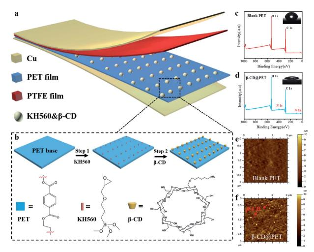
Fig. 1 Schematic diagram of the (a) modified PET based-TENG and (b)  $\beta$ -cyclodextrin ( $\beta$ -CD) modified PET film. The XPS spectrum and contact angle of the (c) blank PET film and (d) modified PET film. AFM photos of the (e) blank PET film and (f) modified PET film.
