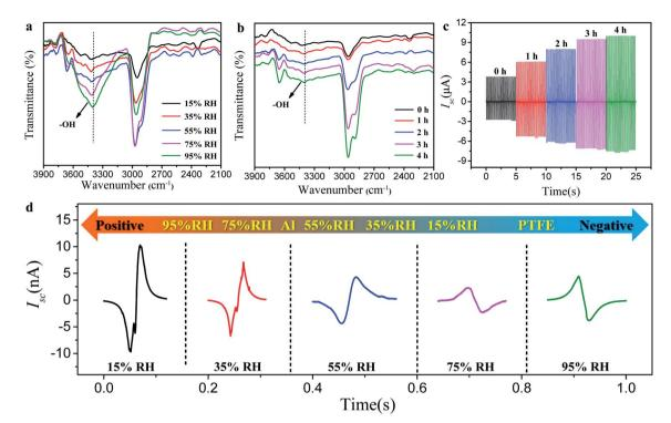
Fig. 5 (a) IR spectra of  $\beta$ -CD@PET films at varying humidities from 15% to 95%, (b) effect of moisture absorption time on IR spectra and (c) output current at 95% humidity for 0 to 5 h, and (d) the value of  $I_{sc}$  and peak shape of the  $\beta$ -CD@PET-Al-based TENG at varying humidities.
