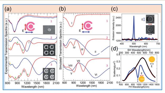
Fig. 8 (a and b) Experimental (a) and calculated (b) transmission spectra of disk (1), SRR (2), and SRR/D (3) arrays.<sup>116</sup> (c and d) Measured SH emission and SH emission intensity versus the incident wavelength (c) and calculated scattering spectra (d) for the single split and perfect nanodisks<sup>119</sup> (reproduced with permission from ref. 116 Copyright 2013 and ref. 119 Copyright 2016, the American Chemical Society).
